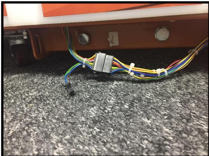
4. Wrap main wires around the plastic hook and connect small wires of the machines with the ones from the wing:
