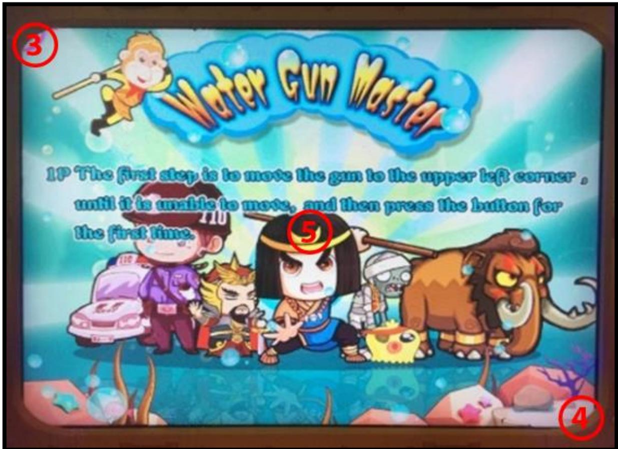
1. Gun (left) will start splashing water. Move the gun to the upper left corner, until is nable to move any further (go to maximum top left) Press middle button once finished.
