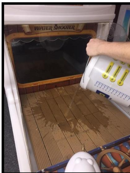
3. If you exceed the limit , the game will stop. Coins will no longer be accepted. A message will appear on the screen: **Beyond the upper water level**. Then, using a for example some cup pour the appropriate amount of water from the water tank.
