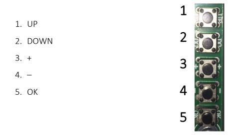
Enter setting mode by pressing OK for 10 seconds.
