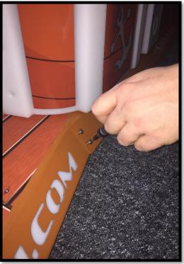
7. Complete joining the wings by putting two small screws at the back of each side:
