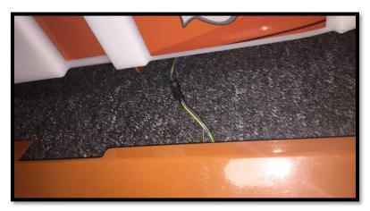
5. RIGHT SIDE ONLY: connect small wires visible on the picture below together:
