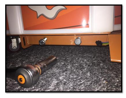
3. LEFT SIDE ONLY: connect main wires visible on the picture below together:
