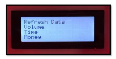
(any data that was set up, changed or adjusted will be loaded onto the game from JM Operator/to JM Operator after pressing chosen button; process takes up to 15 seconds)
